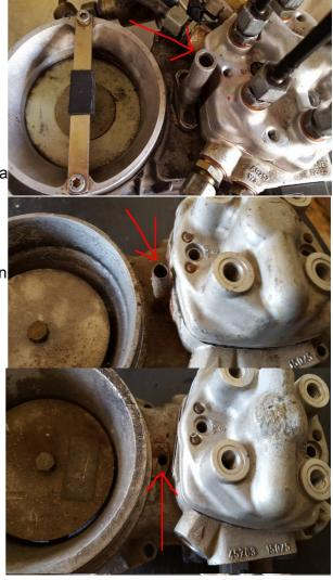
pointing. Turn the key anticlockwise, leaner, until the idle starts to get rough. Make a note of where the key is pointing. Now come to halfway between where the roughness was, then go leaner just slightly. That should be about right.
