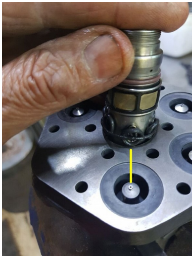
Make sure that the slit is aligned to the outlet jet
