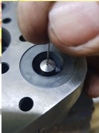
No. 71 drill to ensure the nozzle is clear
