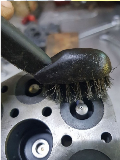
cleaning around the nozzle
