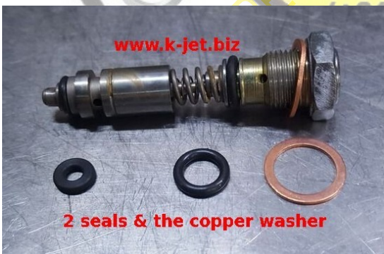
Late System Pressure valve (type 3)
