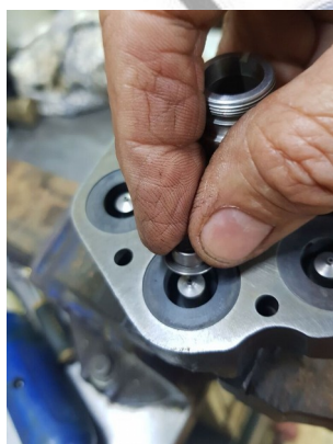
Adjustable type, fit the spring seats, non-adjustable types fit the pressure shim
