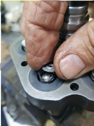
Place the spring caps carefully onto the springs
